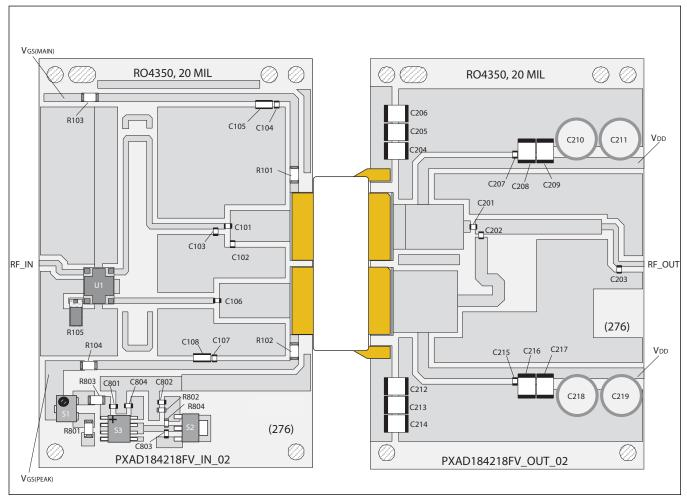
Reference circuit assembly diagram (not to scale)
