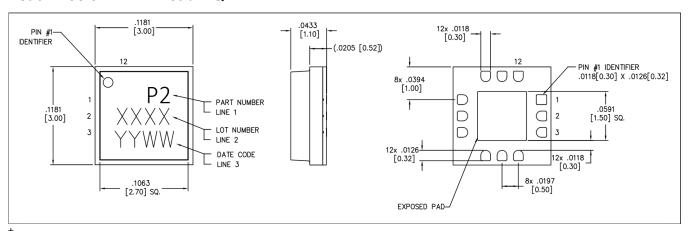
Reference Application Note S2083 for lead-free solder reflow recommendations. Meets JEDEC moisture sensitivity level 3 requirements. Plating is NiPdAu.
