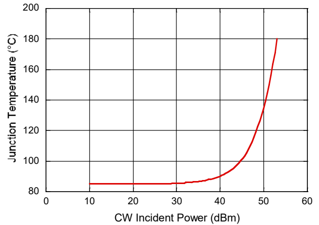
Junction Temperature 1 GHz, CW @ T A = +85°C
