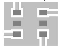
Recommended PCB layout shown above uses 1.6 mm FR4, Grounded coplanar wave guide, transmission line width 0.70 mm and gap 0.57 mm.
