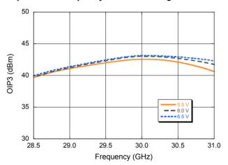
IM3 vs. Frequency over Temperature  $(P_{OUT} = +29 \text{ dBm/Tone})$
