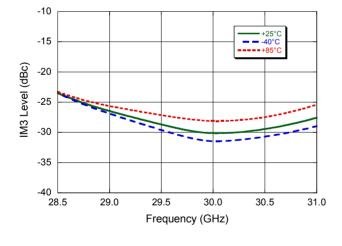
IM3 vs. Frequency over Bias Voltage  $(P_{OUT} = +29 \text{ dBm/Tone})$
