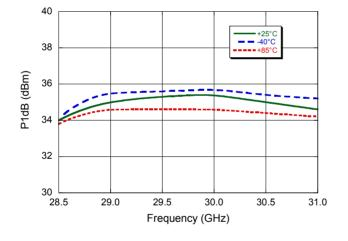
P1dB vs. Frequency over Bias Voltage
