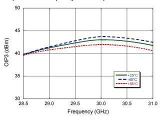
Output IP3 vs. Frequency over Bias Voltage
