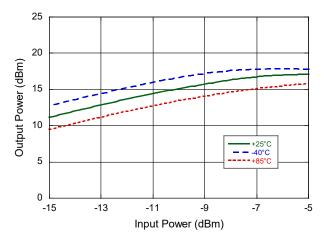
Output Power vs. Input Power @ 42 GHz
