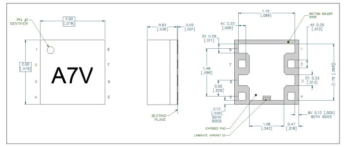
† Reference Application Note S2083 for lead-free solder reflow recommendations. Meets JEDEC moisture sensitivity level 3 requirements. Plating is 100% matte tin over copper.
