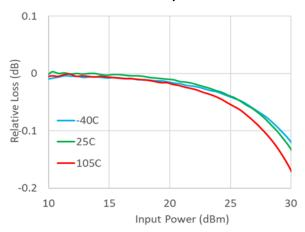
**Evaluation Board Thru Line Insertion Loss**
