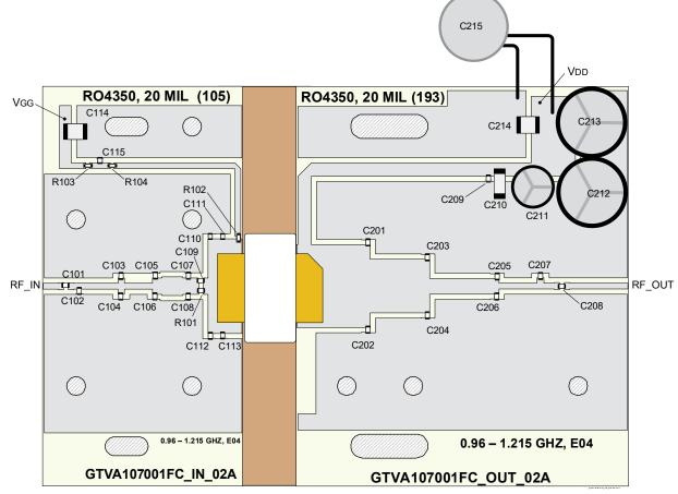
Reference circuit assembly diagram (not to scale)
