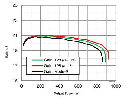
Figure 3. Power Sweep: Gain vs Output Power (Series Show Gain at Various Duty Cycles)  $V_{DS} = 50 \text{ V}, I_{DO} = 100 \text{ mA}, f = 1030 \text{ MHz}$
