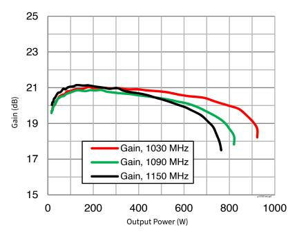
Figure 2. Power Sweep: Gain vs Output Power (Series Show Gain at Frequency)  $V_{_{DS}}$  = 50 V,  $I_{_{DO}}$  = 100 mA, 128 µs Pulse Width, 10% Duty Cycle, Power Optimized
