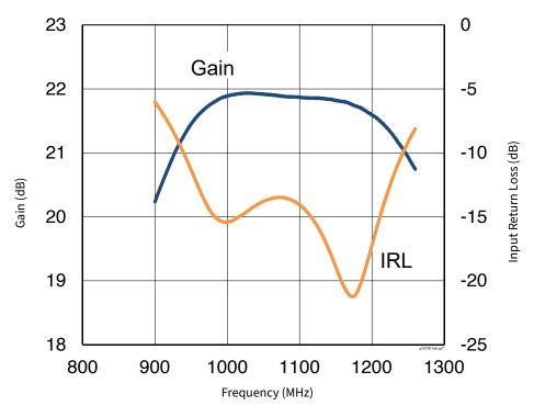
Figure 4. CW Performance Small Signal Gain & Input Return Loss  $V_{_{DD}}$  = 50 V,  $I_{_{DO(MAIN)}}$  = 1000 mA
