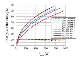
Figure 1. Power Sweep, Pulsed CW  $V_{DS} = 50 \text{ V}$ ,  $I_{DQ} = 100 \text{ mA}$ , 128 µs Pulse Width, 10% Duty Cycle, Power Optimized
