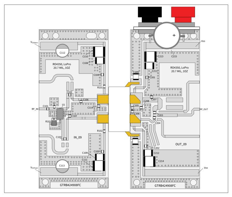
Reference circuit assembly diagram (not to scale)
