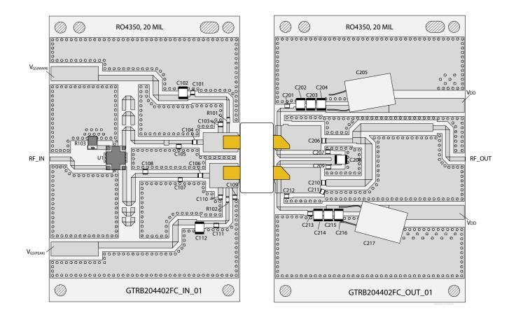
Reference circuit assembly diagram (not to scale)
