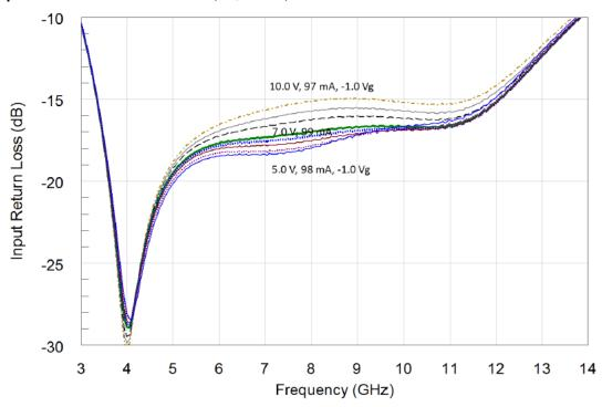
Input Return Loss - Wideband:  $V_D = 5 - 10 \text{ V}$ ;  $V_G = -1 \text{ V}$ ;  $I_D = 99 \text{ to } 97 \text{ mA}$
