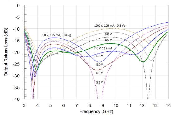
Output Return Loss - Wideband:  $V_D$  = 5 - 10 V;  $V_G$  = -0.8 V;  $I_D$  = 115 to 109 mA
