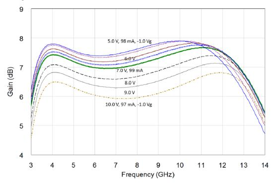
Small Signal Gain - Wideband:  $V_D$  = 5 - 10 V;  $V_G$  = -1 V;  $I_D$  = 99 to 97 mA
