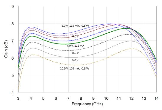
Small Signal Gain - Wideband:  $V_D$  = 5 - 10 V;  $V_G$  = -0.8 V;  $I_D$  = 115 to 109 mA
