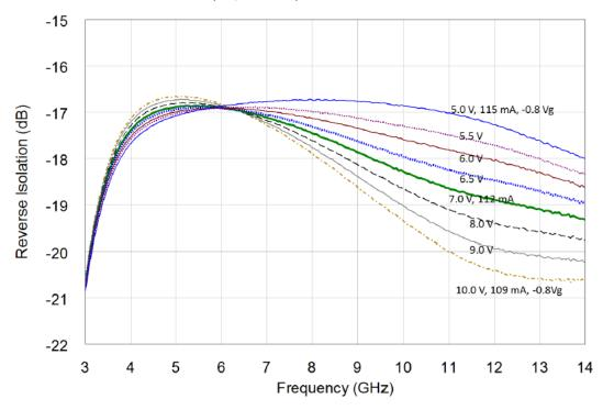
Reverse Isolation - Wideband:  $V_D$  = 5 - 10 V;  $V_G$  = -0.8 V;  $I_D$  = 115 to 109 mA
