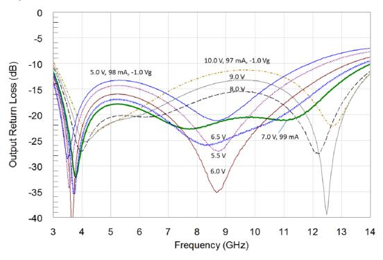
Output Return Loss - Wideband:  $V_D = 5 - 10 \text{ V}$ ;  $V_G = -1 \text{ V}$ ;  $I_D = 99 \text{ to } 97 \text{ mA}$
