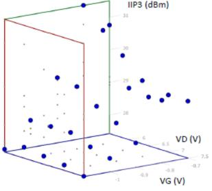
Optimum IIP3 Bias: VD = 5.5 to 6.5 V VG = -0.7 to -0.8 V IIP3 > 30 dBm
