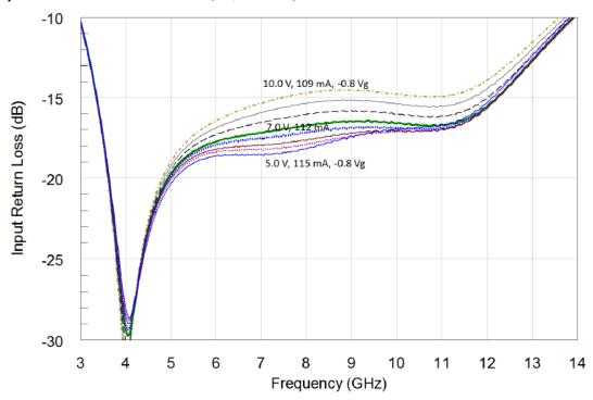
Input Return Loss - Wideband:  $V_D$  = 5 - 10 V;  $V_G$  = -0.8 V;  $I_D$  = 115 to 109 mA
