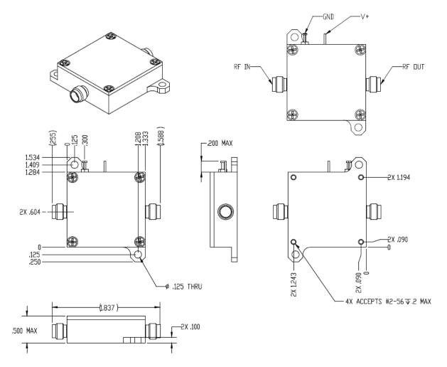
All dimensions are given in inches unless otherwise specified. Typical tolerance: +0.005/-0.005 Mount unit to a low thermal resistance heat sink
