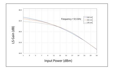
**Figure 25.** Large Signal Gain vs Input Power as a Function of  $I_{DQ}$
