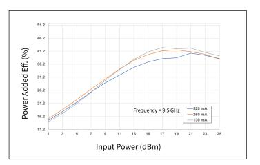
Figure 24. Power Added Eff. vs Input Power as a Function of I<sub>DQ</sub>
