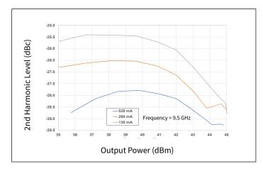
Figure 32. 2nd Harmonic vs Output Power as a Function of I<sub>DO</sub>
