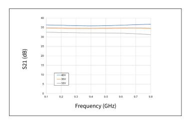
Figure 40. Gain vs Frequency as a Function of Voltage
