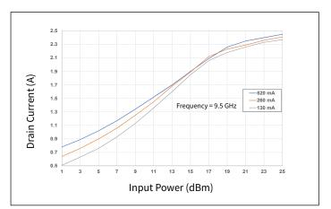
Figure 26. Drain Current vs Input Power as a Function of I<sub>DO</sub>
