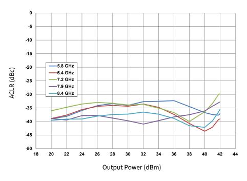
Figure 7. ACLR vs. Output Power and Frequency OQPSK 1.6 Msps  $V_{DD} = 28 \text{ V}, I_{DO} = 285 \text{ mA}$
