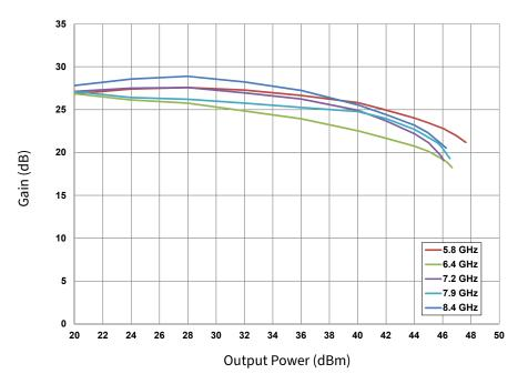
**Figure 12.** Gain vs. Output Power and Frequency  $V_{DD} = 28 \text{ V}$ ,  $I_{DQ} = 800 \text{ mA}$ , Pulsed Width =  $100 \mu s$ , Duty Cycle = 10%
