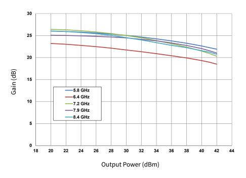
**Figure 5.** Gain vs. Output Power and Frequency OQPSK 1.6 Msps  $V_{DD}$  = 28 V,  $I_{DQ}$  = 285 mA
