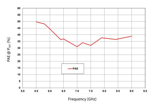
**Figure 9.** Power Added Efficiency @ Saturated Power vs. Frequency  $V_{DD} = 28 \text{ V}$ ,  $I_{DQ} = 800 \text{ mA}$ , Pulsed Width =  $100 \mu s$ , Duty Cycle = 10%
