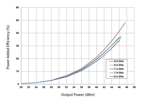
**Figure 11.** PAE vs. Output Power and Frequency  $V_{DD}$  = 28 V,  $I_{DQ}$  = 800 mA, Pulsed Width = 100 $\mu$ s, Duty Cycle = 10%
