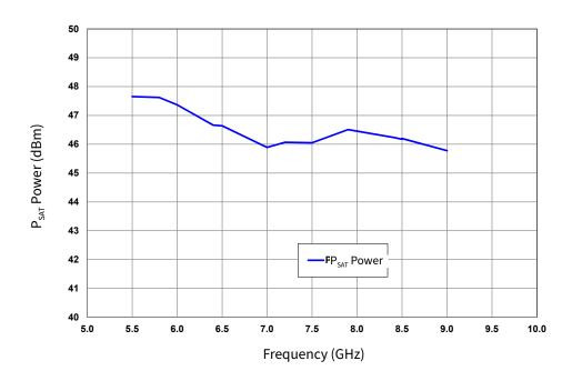
Figure 8. P<sub>SAT</sub> Power vs. Frequency  $V_{DD}$  = 28 V,  $I_{DQ}$  = 800 mA, Pulsed Width = 100 $\mu$ s, Duty Cycle = 10%
