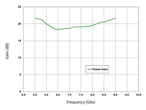
**Figure 10.** Gain @ Saturated Power vs. Frequency  $V_{DD}$  = 28 V,  $I_{DQ}$  = 800 mA, Pulsed Width = 100 $\mu$ s, Duty Cycle = 10%
