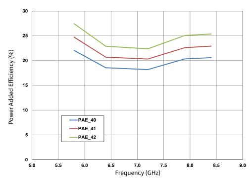
Figure 2. Power Added Efficiency vs. Frequency & Output Power OQPSK  $1.6 \text{ Msps V}_{DD} = 28 \text{ V}, I_{DQ} = 285 \text{ mA}$
