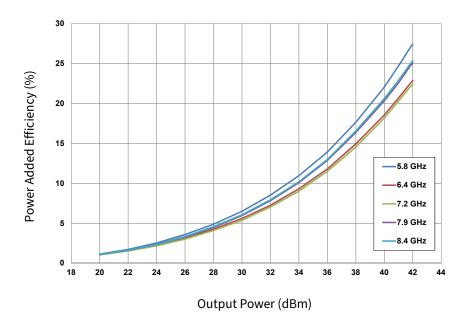
**Figure 6.** Power Added Efficiency vs. Output Power and Frequency OQPSK  $1.6 \text{ Msps V}_{DD} = 28 \text{ V}, I_{DO} = 285 \text{ mA}$
