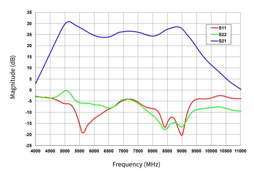
**Figure 4.** Typical S-Parameters  $V_{DD} = 28 \text{ V}$ ,  $I_{DO} = 285 \text{ mA}$
