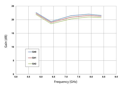
Figure 1. Gain vs. Frequency & Output Power OQPSK 1.6 Msps  $V_{DD} = 28 \text{ V}, I_{DO} = 285 \text{ mA}$
