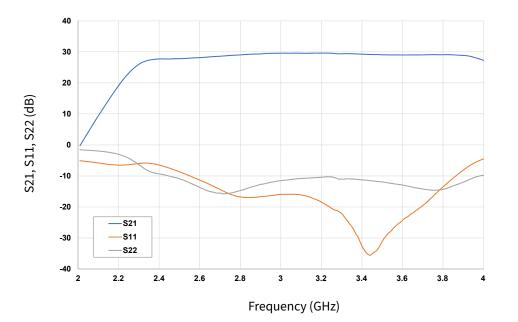
Figure 1. Gain and Return Losses vs Frequency of the CMPA2735075F1 Measured in CMPA2735075F1-AMP Amplifier Circuit  $V_{DS} = 28 V$ ,  $I_{DS} = 800 mA$
