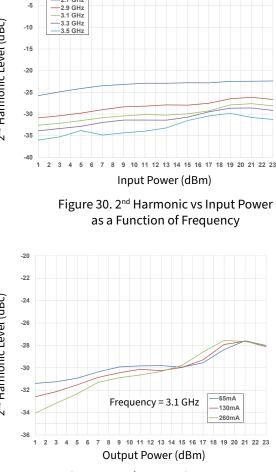
Figure 32. 2<sup>nd</sup> Harmonic vs Output Power as a Function of I<sub>DO</sub>
