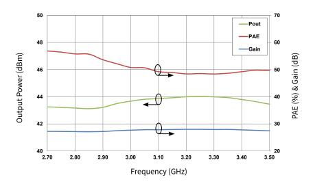
Figure 2. Output Power, Gain and PAE vs Frequency of the CMPA2735015S Measured in CMPA2735015S-AMP1 Amplifier Circuit  $V_{DD} = 50 \text{ V}, I_{DO} = 0.08 \text{ A}, \text{Pulse Width} = 500 \ \mu\text{S}, \text{Duty Cycle} = 10\%$
