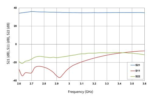
Figure 1. Gain and Input Return Loss vs Frequency in the CMPA2735015S  $V_{DD} = 50 \text{ V}, I_{DQ} = 0.08 \text{ A}$
