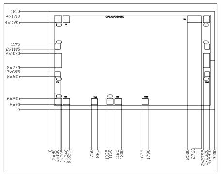
Overall Die Size 2000 X 3000 (+0/-50) Microns, Die Thickness 100 (+/-10) Microns. All Gate and Drain Pads Must be Wire Bonded for Electrical Connection.
