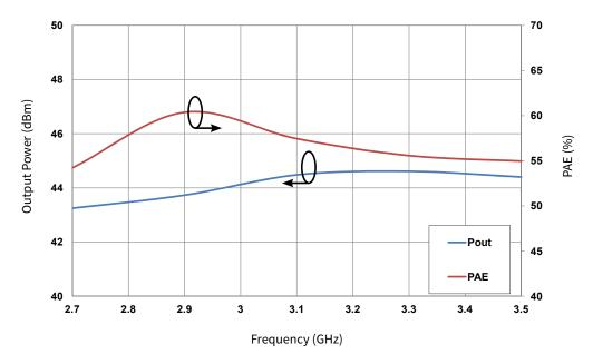
Figure 2. Output Power and PAE vs Frequency in the CMPA2735015S  $V_{DD}$  = 50 V,  $I_{DQ}$  = 0.08 A,  $P_{IN}$  = 16 dBm, Pulse Width = 500  $\mu$ s, Duty Cycle = 10%
