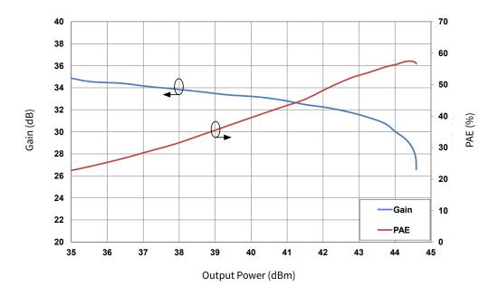
Figure 4. Gain and Power Added Efficiency vs Output Power in the CMPA2735015S  $V_{DD}$  = 50 V,  $I_{DO}$  = 0.08 A, Frequency = 3.1 GHz Pulse Width = 500  $\mu$ s, Duty Cycle = 10%
