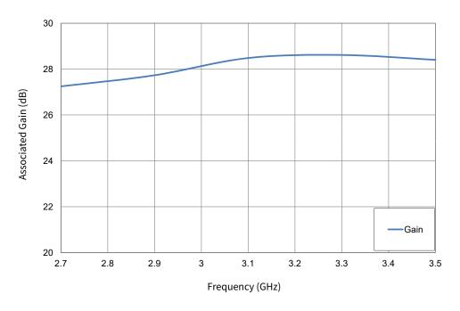
Figure 3. Associated Gain vs Frequency in the CMPA2735015S  $V_{DD}$  = 50 V,  $I_{DO}$  = 0.08 A,  $P_{IN}$  = 16 dBm Pulse Width = 500  $\mu$ s, Duty Cycle = 10%
