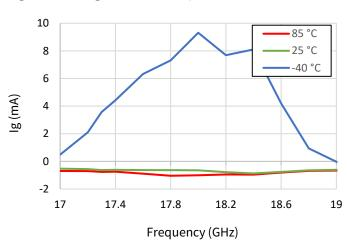
Figure 7: LSG v. Frequency v. Temperature
