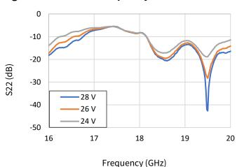
Test conditions unless otherwise noted: Vd=28 V, Idq=0.7A, CW, Pin = -20 dBm, T<sub>base</sub>=25 °C
