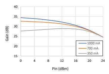
Test conditions unless otherwise noted: Vd=28 V, Idq=0.7A, CW, Pin = -20 dBm, T<sub>base</sub>=25 °C
