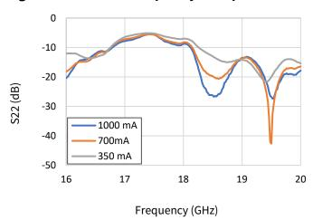
Test conditions unless otherwise noted: Vd=28 V, Idq=0.7A, CW, Pout/tone = 41 dBm, Frequency = 17.8 GHz, Tone Spacing = 1MHz,  $T_{base}$ =25 °C
