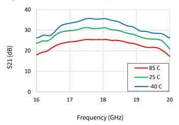
Figure 39: S21 v. Frequency v. Vd
