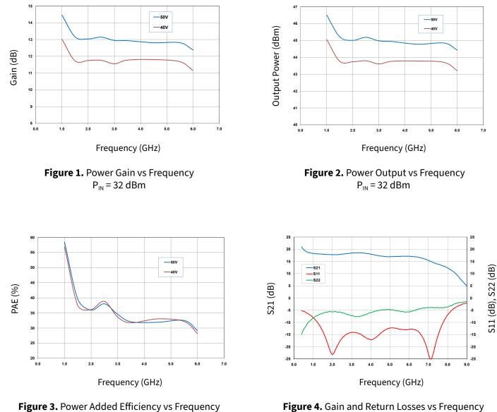
Figure 4. Gain and Return Losses vs Frequency  $V_{DD} = 50 \text{ V}, I_{DO} = 500 \text{ mA}$
