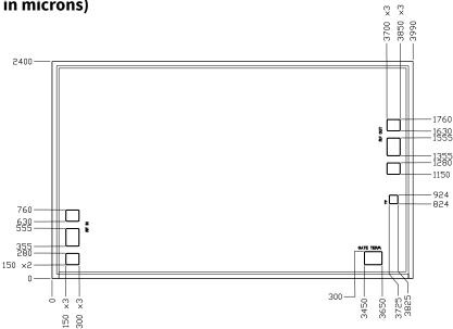
Overall die size 3990 x 2400 (+0/-50) microns, die thickness 100 (+/-10) micron. All Gate and Drain pads must be wire bonded for electrical connection.
