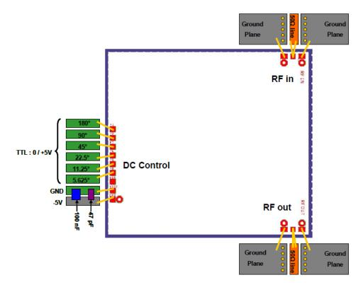
The RF interfacing bond wires or ribbon should be kept as short as possible.
