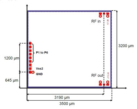
Chip Size =  $3500 \times 3200 \ \mu m$  (including the dicing street) DC Pads =  $100 \times 100 \ \mu m$ , spacing =  $150 \ \mu m$ , top metal = Au RF Pads =  $100 \times 100 \ \mu m$ , pitch =  $150 \ \mu m$ , top metal = Au Chip Thickness =  $100 \ \mu m$
