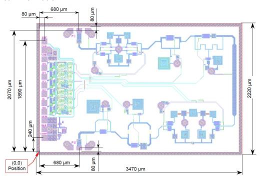
Chip Size = 3470 x 2220  $\mu$ m (± 5  $\mu$ m after dicing) DC Pads = 100 x 100  $\mu$ m, spacing = 150  $\mu$ m, top metal = Au RF Pads = 100 x 100  $\mu$ m, pitch = 150  $\mu$ m, top metal = Au
