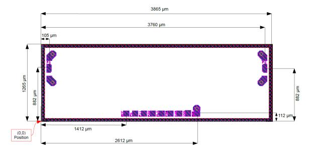
Chip Size =  $3900 \times 1300 \ \mu m \ (\pm 5 \ \mu m)$ DC Pads =  $100 \times 100 \ \mu m$ , spacing =  $150 \ \mu m$ , top metal = Au RF Pads =  $85 \times 150 \ \mu m$ , top metal = Au Chip Thickness =  $100 \ \mu m$
