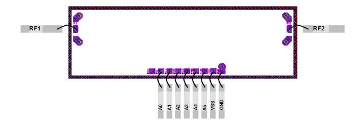
**RF interface** : coplanar or microstrip, bonding  $\approx$  400/500 µm.
