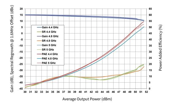
Figure 4. Modulated Power Sweep 1.6 Msps OQPSK Modulation  $V_{DD} = 40 \text{ V}, I_{DO} = 1 \text{ A}, T_{CASE} = 25^{\circ}\text{C}$
