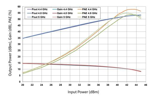
**Figure 10.** Pulsed Power Sweep CGHV50200F in Test Fixture 10% Duty,  $100\mu s$  Pulse Width  $V_{DD} = 40 \text{ V}$ ,  $I_{DQ} = 1 \text{ A}$ ,  $T_{CASE} = 25^{\circ}\text{C}$
