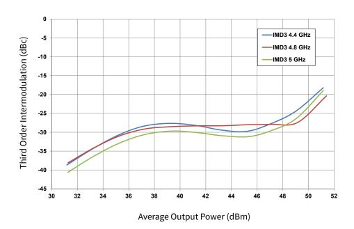
Figure 6. Two Tone Power Sweep IMD3 @ 1 MHz Carrier Spacing  $V_{DD} = 40 \text{ V}, I_{DO} = 1 \text{ A}, T_{CASE} = 25^{\circ}\text{C}$
