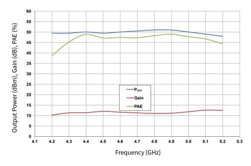
**Figure 2.** Modulated @ Spectral Regrowth = -30dBc, 1.6 MHz from Carrier 1.6 Msps OQPSK Modulation  $V_{DD} = 40 \text{ V}, I_{DO} = 1 \text{ A}, T_{CASE} = 25 ^{\circ}\text{C}$
