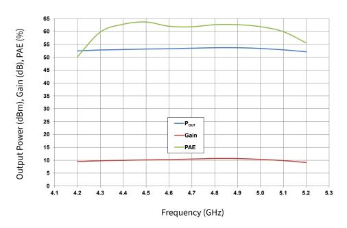
Figure 9. Pulsed vs Frequency @  $P_{IN}$  = 43 dBm CGHV50200F in Test Fixture 10% Duty, 100 $\mu$ s Pulse Width  $V_{DD}$  = 40 V,  $I_{DO}$  = 1 A,  $T_{CASE}$  = 25°C
