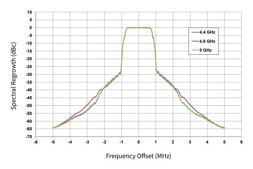
Figure 3. Spectral Mask @ Average Output Power = 48 dBm, 1.6 Msps OQPSK Modulation  $V_{DD} = 40 \text{ V}, I_{DO} = 1 \text{ A}, T_{CASE} = 25^{\circ}\text{C}$
