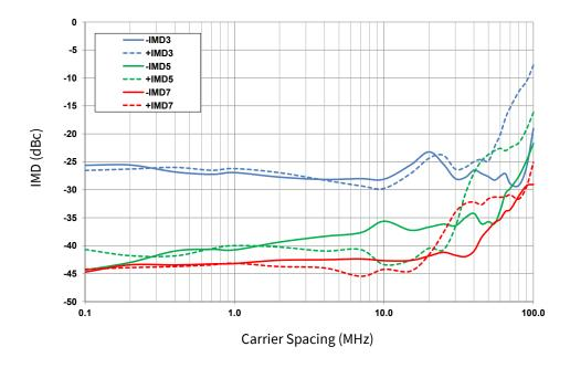
**Figure 8.** Two Tone Carrier Spacing Sweep @ 48 dBm Average Ouput Power, 4.4 GHz  $V_{DD} = 40 \text{ V}, I_{DO} = 1 \text{ A}, T_{CASE} = 25 ^{\circ}\text{C}$
