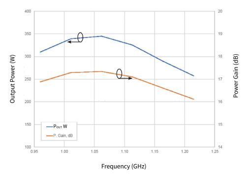
**Figure 8.** Output Power and Power Gain vs. Frequency of the CGHV40180F-AMP3  $V_{DD}$  = 50 V,  $I_{DQ}$  = 1.0 A,  $P_{IN}$  = 38 dBm, 128 µs, 10% pulse
