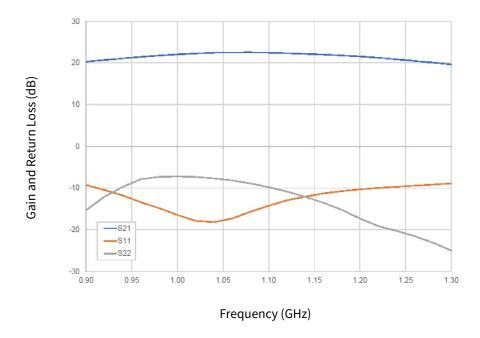
**Figure 6.** Small Signal Gain and Return Losses of the CGHV40180F Measured in Demonstration Amplifier Circuit CGHV40180F-AMP3 CW Operation,  $V_{DD} = 50 \text{ V}$ ,  $I_{DQ} = 1.0 \text{ A}$
