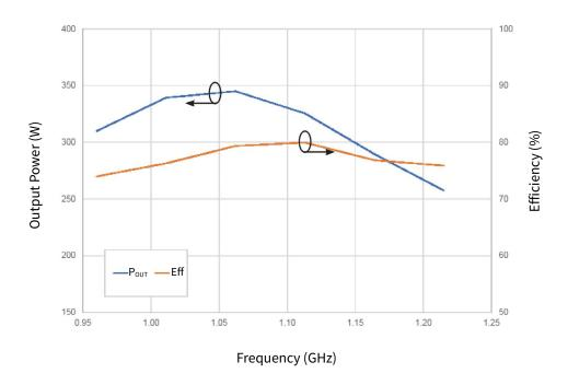
**Figure 7.** Pulsed Output Power and Drain Efficiency vs. Frequency of the CGHV40180F-AMP3  $V_{DD} = 50 \text{ V}$ ,  $I_{DO} = 1.0 \text{ A}$ ,  $P_{IN} = 38 \text{ dBm}$ , 128  $\mu$ s, 10% pulse
