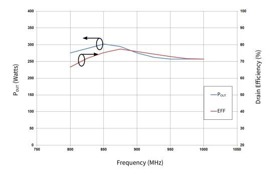
**Figure 2.** Output Power and Drain Efficiency vs Frequency CGHV40180F-TB CW Operation,  $V_{DD} = 50 \text{ V}$ ,  $I_{DQ} = 1.0 \text{ A}$ , @  $P_{IN}$  34 dBm
