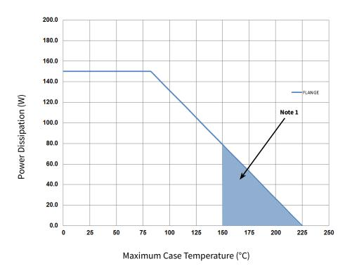
Figure 5. Transient Power Dissipation De-rating Curve
