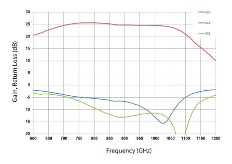
Figure 1. Small Signal Gain and Return Loss versus Frequency measured in application circuit CGHV40180F  $V_{DD} = 50 \text{ V}, I_{DO} = 1.0 \text{ A}$
