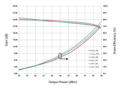
**Figure 3.** Gain and Drain Efficiency vs. Frequency and Output Power CGHV40180F-TB CW Operation,  $V_{DD} = 50 \text{ V}$ ,  $I_{DQ} = 1.0 \text{A}$
