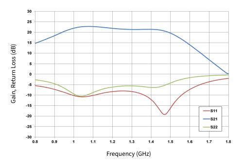
Figure 1. Typical Small Signal Response of CGHV40030-AMP Application Circuit  $V_{DD} = 50 \text{ V}, I_{DQ} = 150 \text{ mA}$
