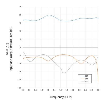
**Figure 3.** Typical Small Signal Response of CGHV40030F-AMP2  $V_{DD} = 50 \text{ V}, I_{DO} = 90 \text{ mA}$
