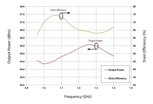
**Figure 2.** Typical Large Signal Response of CGHV40030-AMP Application Circuit  $V_{DD} = 50 \text{ V}$ ,  $I_{DO} = 150 \text{ mA}$ ,  $P_{IN} = 29 \text{ dBm}$ ,  $T_{CASE} = 25^{\circ}\text{C}$ , CW
