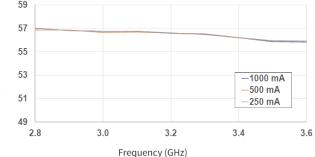
Drain Efficiency vs. Frequency over IDQ
