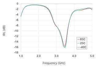
Output Return Loss vs. Frequency over Temperature
