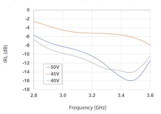
Output Return Loss vs. Frequency over Voltage
