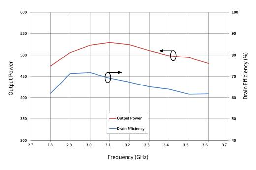
Figure 2. CGHV35400F  $P_{OUT}$  and Drain Efficiency vs Frequency at  $T_{case}$  = 25 °C  $V_{DD}$  = 50 V,  $I_{DQ}$  = 0.5 A,  $P_{IN}$  = 46 dBm, Pulse Width = 500  $\mu$ s, Duty Cycle = 10%
