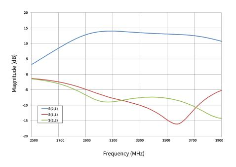
Figure 1. CGHV35400F Typical S Parameters  $V_{DD}$  = 50 V,  $I_{DQ}$  = 0.5 A
