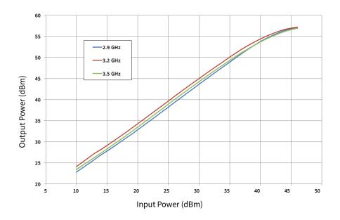
Figure 3. CGHV35400F Output Power vs Input Power V  $_{DD}$  = 50 V, I  $_{DQ}$  = 500 mA, Pulse Width = 500  $\mu s$ , Duty = 10%, T  $_{case}$  = 25 °C
