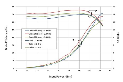
Figure 4. CGHV35400F Drain Efficiency & Gain vs Input Power  $V_{DD}$  = 50 V,  $I_{DQ}$  = 500 mA, Pulse Width = 500  $\mu$ s, Duty Cycle = 10%,  $T_{case}$  = 25 °C
