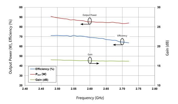
**Figure 2.** Gain, Output Power, and Drain Efficiency under 100µs Pulse Width, 10% Duty Cycle for the CGHV27060MP Measured in Demonstration Amplifier Circuit CGHV27060MP-AMP1
