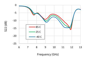
Figure 43: S22 v. Frequency v. Vd
