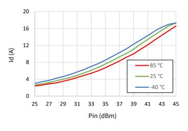
Figure 26: Ig v. Pin v. Temperature
