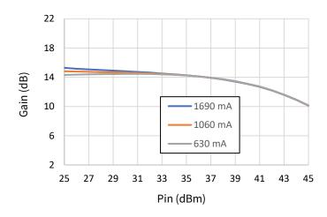
Test conditions unless otherwise noted: Vd=45V, Idq= 1060mA, Signal = CW, Pin = -20dBm, T<sub>base</sub>=25 °C
