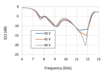
Test conditions unless otherwise noted: Vd=45V, Idq=1060mA, Signal = CW, Pin = -20dBm, T<sub>base</sub>=25 °C
