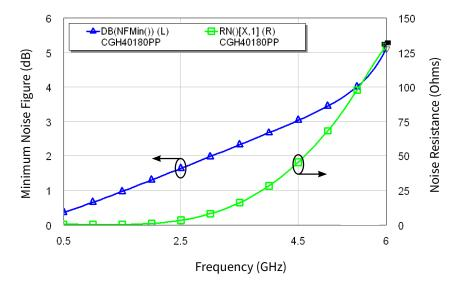
Figure 5. Simulated Minimum Noise Figure and Noise Resistance vs Frequency of the CGH40180PP  $V_{DD}$  = 28 V,  $I_{DQ}$  = 1 A
