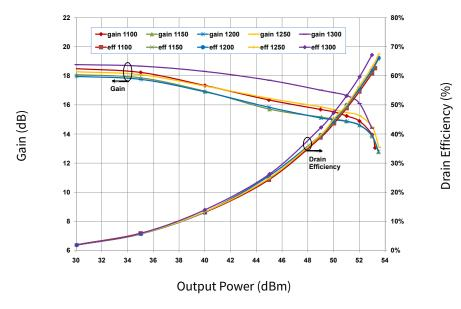
Figure 3. Gain and Drain Efficiency vs Output Power measured in Broadband Amplifier Circuit CGH40180PP-AMP  $V_{DD} = 28 \text{ V}, \text{ I}_{DQ} = 2.0 \text{ A}$
