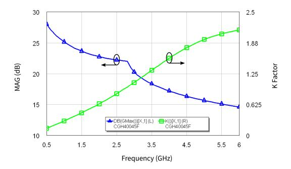
**Figure 7.** Simulated Maximum Available Gain and K Factor of the CGH40045  $V_{DD}$  = 28 V,  $I_{DQ}$  = 400 mA
