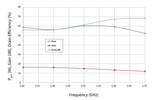
Figure 2. Gain, Efficiency, and Output Power vs Frequency measured in Amplifier Circuit CGH40045F-AMP  $V_{DD}=28\ V,\ I_{DO}=400\ mA$
