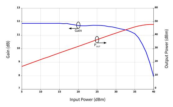
**Figure 5.** Pulsed Gain and Output Power vs Input Power measured in Amplifier Circuit CGH40045F-AMP  $V_{DD} = 28 \text{ V}, I_{DO} = 800 \text{ mA}, Freq = 3.6 \text{ GHz}, Pulse Width = 200 \mu S, 10\% \text{ Duty Cycle}$
