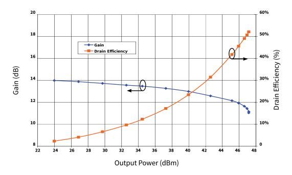
Figure 3. Gain and Efficiency vs Output Power measured in Amplifier Circuit CGH40045F-AMP  $V_{DD} = 28 \text{ V}, I_{DO} = 400 \text{ mA}, \text{Freq} = 2.5 \text{ GHz}$
