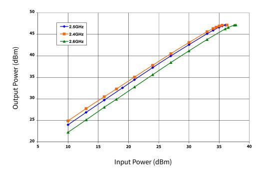
Figure 4. Single Tone CW Output Power vs Input Power measured in Amplifier Circuit CGH40045F-AMP  $V_{DD} = 28 \text{ V}, I_{DO} = 400 \text{ mA}$
