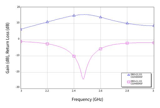
Figure 1. Simulated Small Signal Gain and Input Return Loss of the CGH40045F-AMP vs Frequency  $V_{DD} = 28 \text{ V}, I_{DO} = 400 \text{ mA}$
