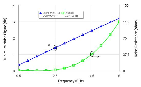
Figure 8. Simulated Minimum Noise Figure and Noise Resistance vsFrequency of the CGH40045  $V_{DD} = 28 \text{ V}, I_{DO} = 400 \text{ mA}$
