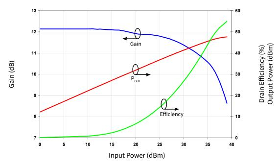
**Figure 6.** Single Tone CW Gain, Efficiency, and Output Power vs Input Power measured in Amplifier Circuit CGH40045F-AMP  $V_{DD} = 28 \text{ V}, I_{DO} = 800 \text{ mA}, \text{Freq} = 3.6 \text{ GHz}$
