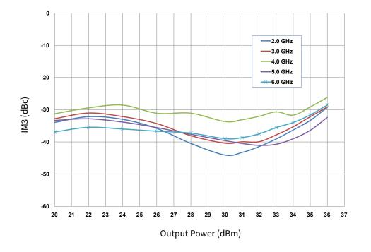
Figure 10. Third Order Intermodulation Distortion vs Average Output Poweras a Function of Frequency of the CGH40006S in the CGH40006S-AMP1  $V_{DD} = 28 \text{ V}, I_{DQ} = 60 \text{ mA}$
