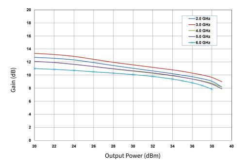
Figure 3. Power Gain vs Output Power as a Function of Frequency of the CGH40006S in the CGH40006S-AMP1  $V_{DD} = 28 V$ ,  $I_{DO} = 100 mA$
