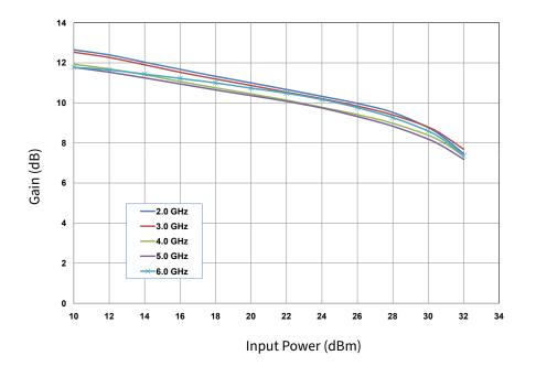
Figure 5. Power Gain vs Input Power as a Function of Frequency of the CGH40006S in the CGH40006S-AMP1  $V_{DD}$  = 28 V,  $I_{DQ}$  = 100 mA
