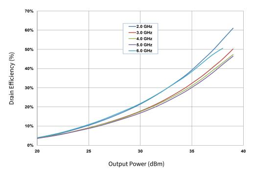
Figure 6. Drain Efficiency vs Output Power as a Function of Frequency of the CGH40006P in the CGH40006P-AMP  $V_{DD} = 28 \text{ V}, I_{DQ} = 100 \text{ mA}$
