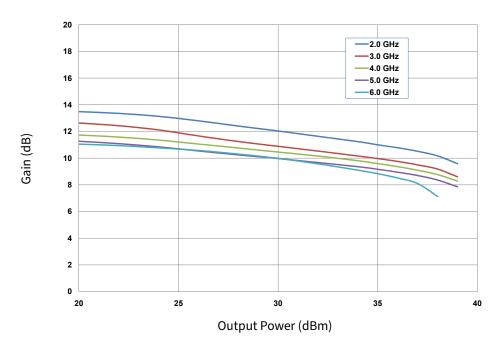
Figure 5. Power Gain vs Output Power as a Function of Frequency of the CGH40006P in the CGH40006P-AMP  $V_{DD} = 28 \text{ V}, I_{DO} = 100 \text{ mA}$
