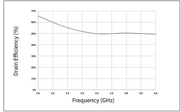
Figure 11. Drain Efficiency vs Frequency of the CGH40006P in the CGH40006P-AMP  $P_{IN} = 32 \text{ dBm}, V_{DD} = 28 \text{ V}$
