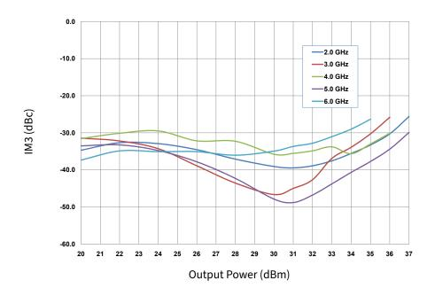
Figure 13. Third Order Intermodulation Distortion vs Average Output Power as a Function of Frequency of the CGH40006P in the CGH40006P-AMP  $V_{DD} = 28 \text{ V}$ ,  $I_{DO} = 60 \text{ mA}$
