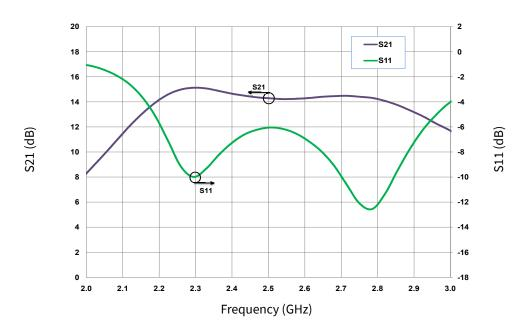
Figure 1. Gain and Return Loss vs Frequency measured in Broadband Amplifier Circuit CGH27060F-AMP  $V_{DD} = 28 \text{ V}, I_{DQ} = 300 \text{ mA}$
