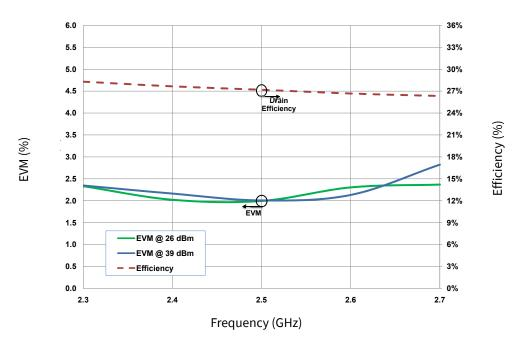
**Figure 2.** Typical EVM at 24 dBm and 39 dBm vs Frequency measured in Broadband Amplifier Circuit CGH27060F-AMP
