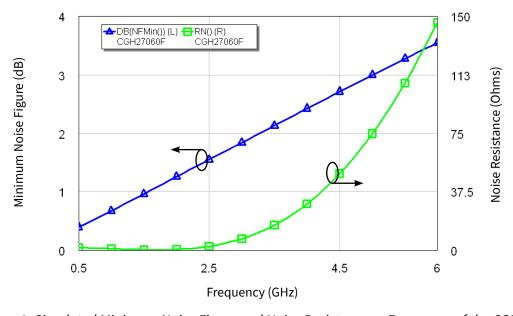
Figure 6. Simulated Minimum Noise Figure and Noise Resistance vs Frequency of the CGH27060  $V_{DD} = 28 \text{ V}, I_{DQ} = 100 \text{ mA}$
