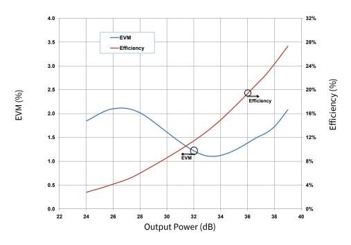
Figure 3. Drain Efficiency and EVM vs Output Power measured in CGH27060F-AMP  $V_{DD} = 28 \text{ V}, I_{DQ} = 300 \text{ mA}, 802.16-2004 \text{ OFDM}, PAR = 9.8 \text{ dB}$
