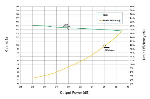
Figure 4. Typical Gain and Efficiency vs Output Power measured in CGH27060F-AMP  $V_{DD} = 28 \text{ V}, I_{DQ} = 300 \text{ mA}, 802.16-2004 \text{ OFDM}, PAR = 9.8 \text{ dB}$
