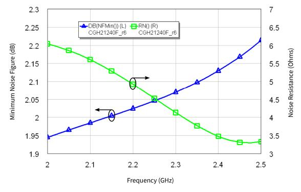
Figure 9. Simulated Minimum Noise Figure and Noise Resistance vs Frequency of the CGH21240F  $V_{DD} = 28 \text{ V}, I_{DO} = 1.0 \text{ A}$
