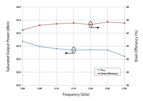
**Figure 2.** Typical Pulsed Saturated Power and Drain Efficiency vs Frequency of the CGH21240F measured in CGH21240F-AMP Amplifier Circuit.  $V_{DS} = 28 \text{ V}$ ,  $I_{DS} = 1.0 \text{ A}$ ,  $P_{SAT} = 20 \text{ mA } I_{GS}$  Peak, Pulse Width =  $40 \mu s$ , Duty Cycle = 5 %
