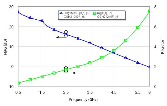
Figure 8. Simulated Maximum Available Gain and K Factor of the CGH21240F  $V_{DD}$  = 28 V,  $I_{DO}$  = 1.0 A
