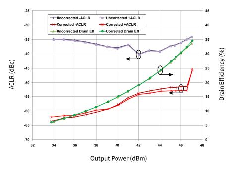
Figure 5. WCDMA Characteristics with and without DPD Correction ACLR and Drain Efficiency vs Output Powerof the CGH21240F measured in CGH21240F-AMP Amplifier Circuit  $V_{DS} = 28 \text{ V}, I_{DS} = 1.0 \text{ A}, \text{Frequency} = 2.14 \text{ GHz}$
