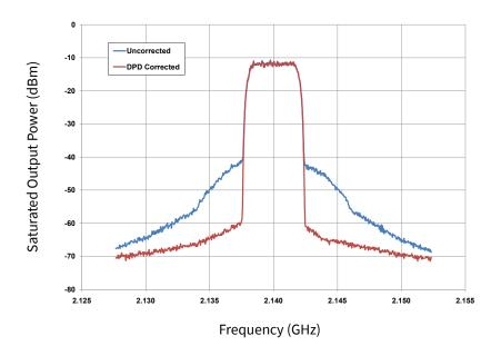
**Figure 6.** WCDMA Linearity with DPD Linearizer of the CGH21240F measured in CGH21240F-AMP Amplifier Circuit Single Channel WCDMA 6.5dB PAR with CFR  $V_{DS} = 28 \text{ V}$ ,  $I_{DS} = 1.0 \text{ A}$ ,  $P_{AVE} = 46 \text{ dBm}$ , Efficiency = 30%
