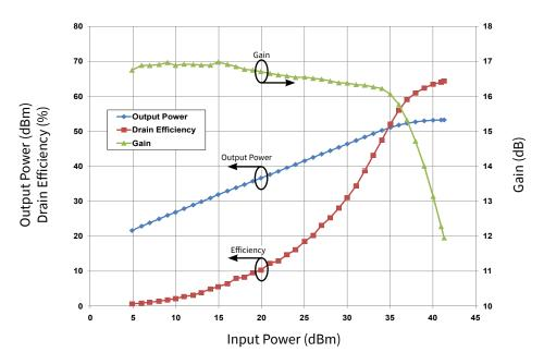
**Figure 1.** Typical Pulsed Output Power, Drain Efficiency, and Gain vs Input Power of the CGH21240F measured in CGH21240F-AMP Amplifier Circuit  $V_{DS} = 28 \text{ V}$ ,  $I_{DS} = 1.0 \text{ A}$ , Freq = 2.14 GHz, Pulse Width = 40 $\mu$ s, Duty Cycle = 5%
