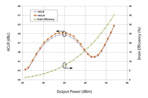
**Figure 4.** Typical WCDMA Characteristics ACLR and Drain Efficiency vs Output Power of the CGH21240F measured in CGH21240F-AMP Amplifier Circuit 3GPP Test Model 1, 64 DPCH, 67% Clipping, 8.81 dB PAR @ 0.01%  $V_{DS} = 28 \text{ V}$ ,  $I_{DS} = 1.0 \text{ A}$ , Frequency = 2.14 GHz
