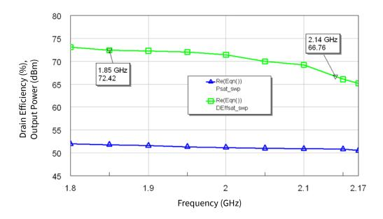
Figure 7. Simulated Performance of the CGH21240F from 1.8 - 2.17 GHz  $V_{DD} = 28 \text{ V}, I_{DO} = 1.0 \text{ A}$
