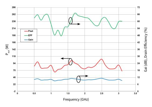
Figure 2. Output Power and Efficiency of the CG2H30070F vs Frequency as Measured in the Single-ended Demonstration Amplifier CG2H30070F-AMP CW Operation,  $V_{DD} = 28 \text{ V}$ ,  $I_{DO} = 1.0 \text{ A}$ ,  $P_{IN} = 39 \text{ dBm}$
