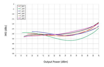
Figure 6. IM3 vs Output Power of the CG2H30070F as Measured in the Single-ended Demonstration Amplifier CG2H30070F-AMP  $I_{DQ}=1000~\text{mA}, \text{Temperature}=25~^{\circ}\text{C}$
