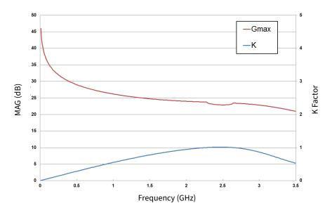
Figure 4. Simulated Maximum Available Gain and K-factor of the CG2H30070F  $\rm V_{DD}$  = 28 V,  $\rm I_{DO}$  = 1.0 A
