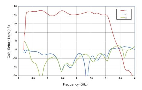
Figure 1. Small Signal Gain and Return Losses of the CG2H30070F vs Frequency as Measured in the Single-ended Demonstration Amplifier CG2H30070F-AMP  $\rm V_{DD}=28~V,~I_{DQ}=1.0~A$
