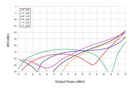
Figure 5. IM3 vs Output Power of the CG2H30070F as Measured in the Single-ended Demonstration Amplifier CG2H30070F-AMP  $I_{_{\rm DO}}=300~{\rm mA, Temperature}=25~{\rm ^{\circ}C}$
