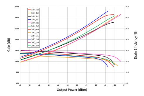
Figure 3. Gain and Drain Efficiency vs Output Power at Various Frequencies as Measured in the Single-ended Demonstration Amplifier CG2H30070F-AMP CW-Operation,  $V_{DD} = 28 \text{ V}$ ,  $I_{DO} = 1.0 \text{ A}$
