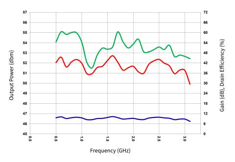
Figure 8. Output Power, Power Gain, and Drain Efficiency vs Frequency of Two CG2H30070F Combined as Measured in the Combined Demonstration Amplifier CG2H30070F-AMP2 with Couplers  $V_{DD} = 28 \text{ V}, I_{DO} = 2 \text{ A}, P_{IN} = 42.5 \text{ dBm}, Temperature = 25 °C$
