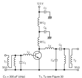
$L_2 = 4.2 \text{ nH (adjust)}$   $L_3 = 8 \text{ nH (adjust)}$   $C_4 = 130 \text{ pF (chip)}$  $C_5 = 750 \text{ pF (chip)}$
