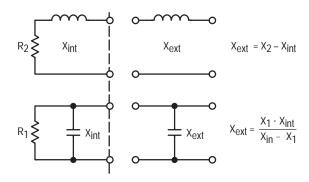
Figure 6. Termination Reactance Compensation
