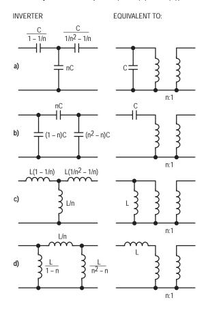
Figure 26. Impedance Inverters
