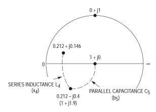
Figure 36. Output Circuit Design
