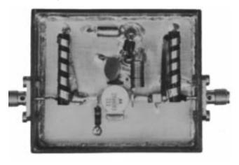
118 – 136 MHz Amplifier (see Figure 37) Before Coil Adiustment
