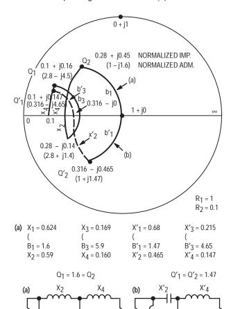
Figure 13. Transformation Paths for Networks (a) and (b)
