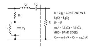
Figure 27. Roll-Off Compensation Network
