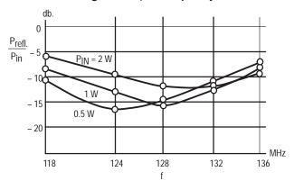
Figure 40. PREFL./PIN vs Frequency
