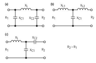
Figure 9. Three-Reactance Matching Networks
