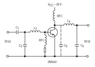
Figure 33. Narrow-Band VHF Power Amplifier
