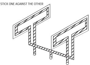
Figure 29. 4:1 Line Transformer on P.C. Board
