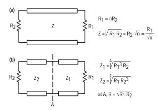
Figure 18. Transformation Networks Using  $\lambda$ /4-Long Transmission Lines
