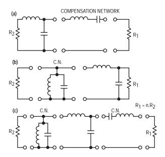
Figure 16. Compensation Networks Used with a L-Section
