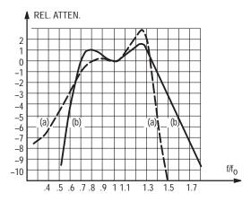
Figure 15. Selectivity curves for networks (a) and (b) of Figure 13 with Infinite R<sub>1</sub>
