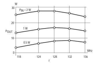
Figure 38. POUT vs Frequency
