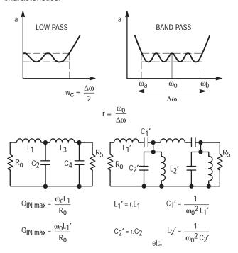
Figure 25. Conversion from Low-Pass into Band-Pass Filter
