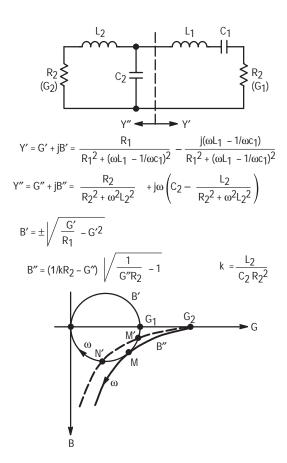
Figure 17. Y-Plane Representation of the Circuit of Figure 16(a)
