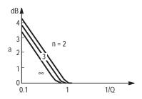
Figure 24. Insertion Losses as a Function of 1/Q
