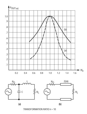
Figure 8. Bandwidth of the L-Section for n = 10 (a) with Lumped Constants (b) with a Transmission Line ( $\lambda$ /4)
