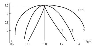
Figure 20. Selectivity Curves for One, Two and Three  $\lambda$ 4-Sections
