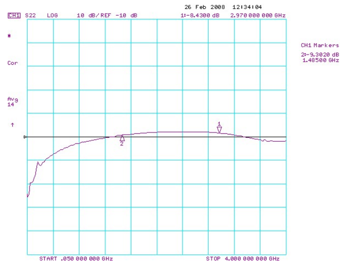
Figure 13. S_{22} = -8.4\text{dB} @ 3 GHz, with 0dB output attenuator, L_{\text{match}} = 2.7\text{nH}
