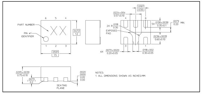
Reference Application Note S2083 for lead-free solder reflow recommendations. Meets JEDEC moisture sensitivity level 1 requirements. Plating is 100% matte tin over copper.
